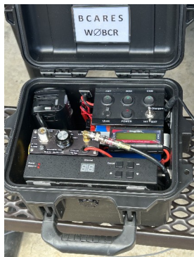
BCARES, 70cm, 3W, DVB-T Transmitter
