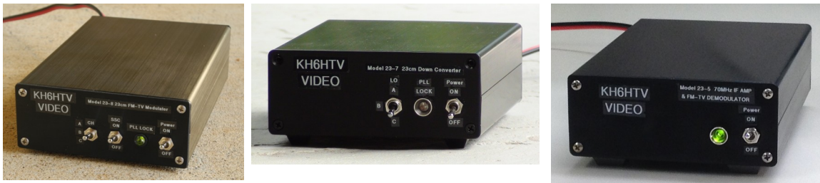
Fig. 21 KH6HTV Video FM-TV products 23cm modulator (left), 23cm down-converter (middle) and 70 MHz IF & Demodulator (right)
