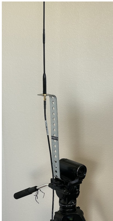
Fig. 20 70 cm & 23 cm flexible whip HT antenna. Diamond SRH-999 1.7 dBi on 70 cm & 3.2 dBi on 23 cm bands mounted on camera tripod along with Canon camcorder
