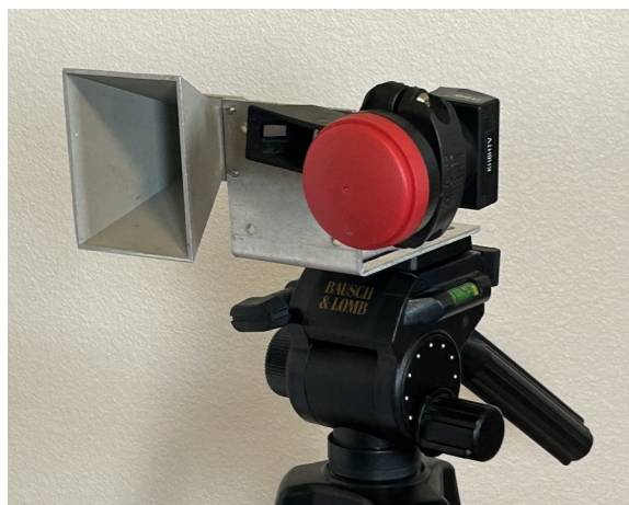
Fig. 18 X-band, 3 cm Waveguide horn antenna (17dBi) used for transmit and BullsEye LNB (14.6dBi) used for receive
