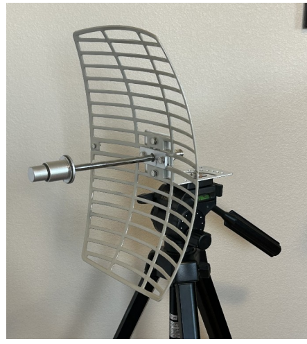
Fig. 19 23 cm, 14 dBi patch antenna --- 9 cm, 15 dBi patch antenna, & 5 cm, 22 dBi BBQ grill dish antenna
