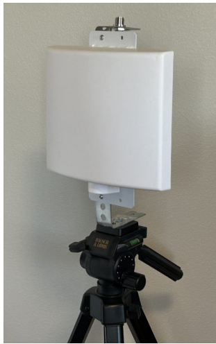
Fig. 19 23 cm, 14 dBi patch antenna --- 9 cm, 15 dBi patch antenna, & 5 cm, 22 dBi BBQ grill dish antenna
