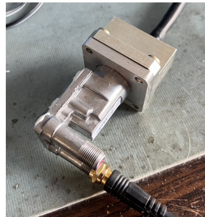
X band wave guide transition to Bulls Eye LNB for testing
